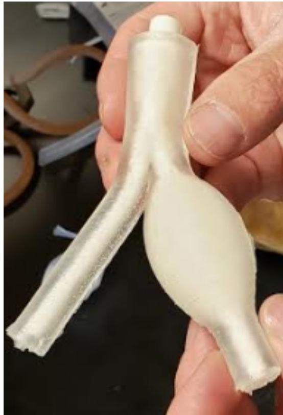
Figure 24: Prototype Iliac Bifurcation Model Proving a Successful Manufacturing Process
